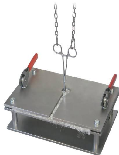
Item no.: THS1067-10 Fixture to test tuft withdrawal force for carpets according to ISO 4919, incl. surgical forceps
