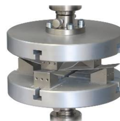
THS1498-8P-200-CR2 8-point bend test fixture for metal sheets
