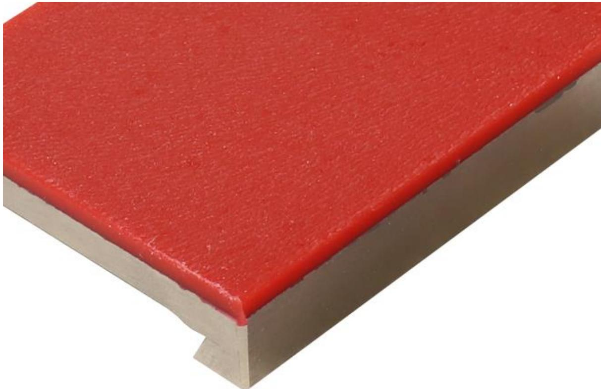
Vulkollan® is a high-performance polyurethane elastomer originally developed by Bayer AG (now Covestro). It is well-known for its outstanding mechanical properties, making it one of the toughest and most versatile synthetic elastomers in industrial applications. Composed primarily of Desmodur® 15 (a special NDI-based isocyanate) and polyester-polyols, Vulkollan undergoes a complex, closely controlled hot-casting process to achieve its distinctive characteristics.
